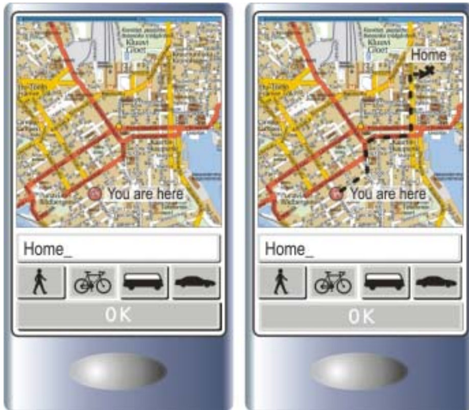
Fig. 1. A handheld route guide that finds the best route by walking, bike, public transportation or car. The system recognizes the user's current location. The user needs to determine the destination and the form of moving.
