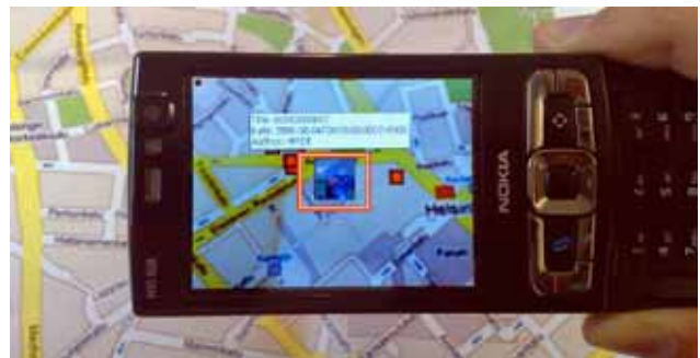
Figure 1. MapLens in use with a paper map, overlaying digital information on screen. The red square (centre) is used to select markers.
