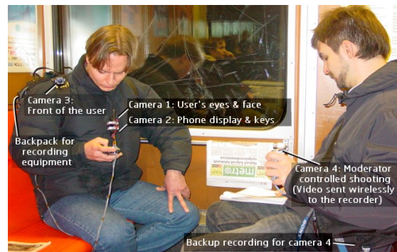
Figure 2. Configuration of recording equipment.
