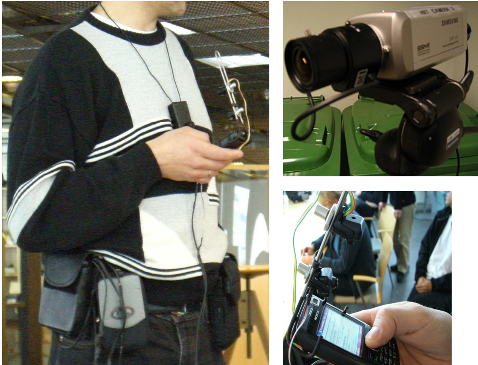
Figure 4. Version 2 of Figure 1’s mobile video recording system. Some characteristics: (a) All noncamera equipment except cables fit on a belt and weigh less than 2 kilograms in total; (b) Environmental cameras can be switched to on the fly, based on signal strength; (c) All video and audio inputs are integrated on the fly to a four-video display; (d) The cameras are flexible, can be worn or attached to the mobile device, and can operate with cables or wirelessly; (e) There is an option for remotely triggered recording events initiated via Bluetooth; (f) Operational duration is up to 4 hours without battery change or other maintenance operations.
