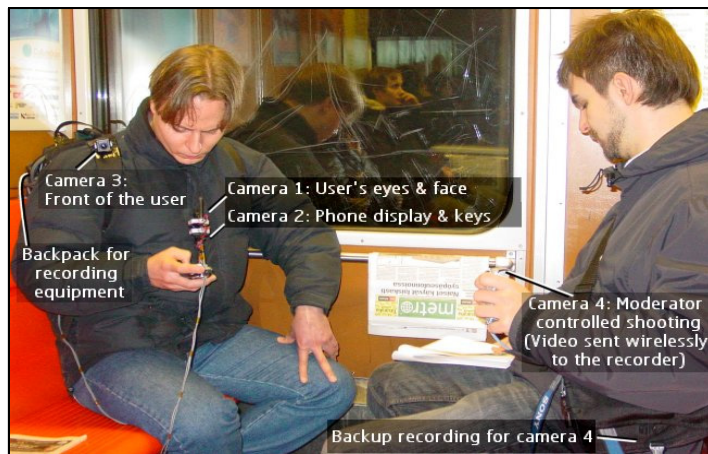
Figure 1. Two setups for experimentation in HCI. On the top, Jakob Nielsen’s (1995) laboratory setup at Sun Microsystems that worked as a model and baseline for many laboratories built around the world in the 1990s. On the bottom, one of the first published “mobile usability labs,” developed in joint effort between Nokia Research Center and HIIT (Roto et al., 2004).
