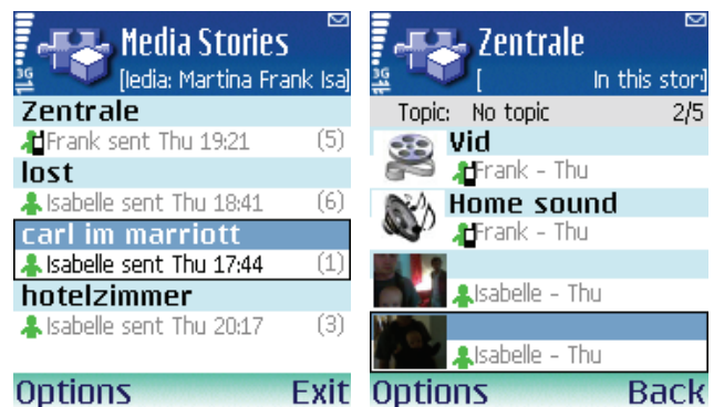
Figure 3. CoMedia's view to Media Stories (on left). Upon selecting a Story, the user can see media in that Story. Awareness cues indicate whether other users are online and if they in proximity versus distant.
