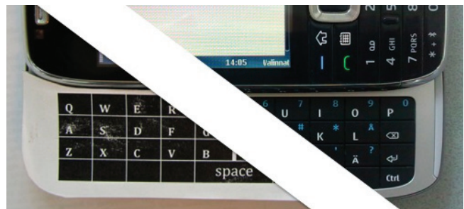
Figure 3. A thin layer of plastic on the keyboard (left) was used to block feedback from the button edges and key releases of the original keyboard (right). Keymaps were printed on top of this layer (physical-QWERTY input shown here).
