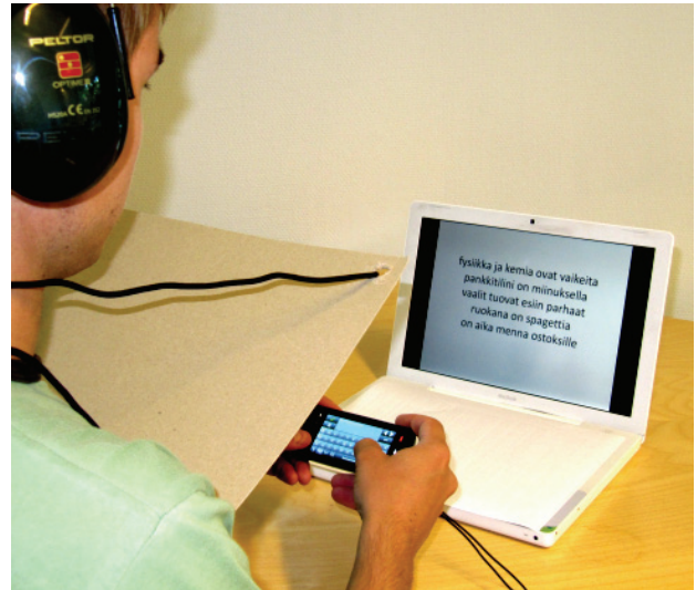
Figure 1. A user in the t condition—tactile feedback unblocked and vision (cardboard) and audition (ear protection) blocked.
