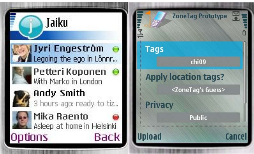
Fig 1. Left: Jaiku shows contacts' presence lines and real-time location cues. Right: ZoneTag's automation suggests tags to be added to photos.
